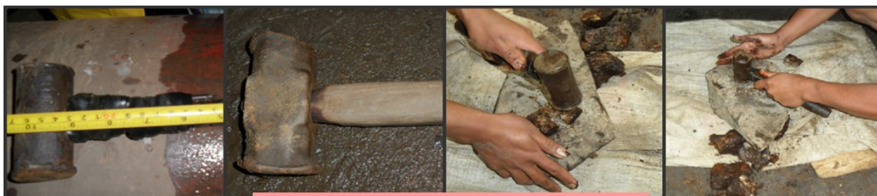
Hammer “maso” used in crushing ores
